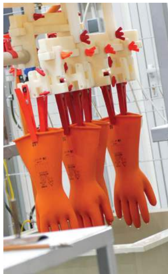
SPH-O Testing stand for Insulator Covers
