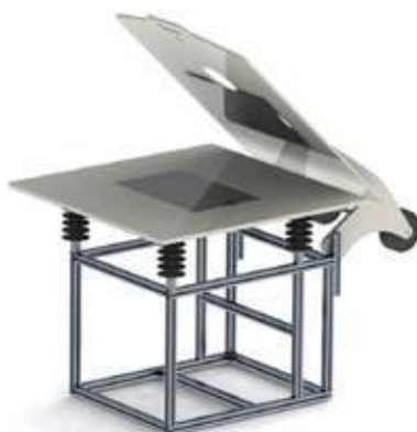
Testing Stand for Insulating Blankets and Mats
