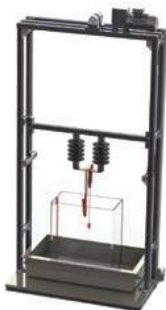
SPH-SOI Testing Stand for Personal Protective Equipment - Electrical Insulating Sleeves
